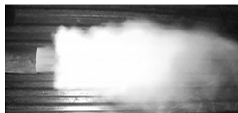
Figure 2. Pulsed detonation steam superheater (left) and its pulsed USS exhaust plume (right).
